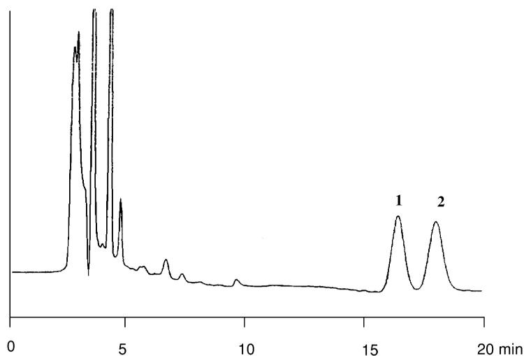
Fig. 2. Separation of the (1) (+)- and (2) (-)-nisoldipine enantiomers (1  $\mu\text{g}$  of rac-nisoldipine/ml solution) by HPLC on a Chiralcel<sup>®</sup> OD-H column with the mobile phase consisting of an *n*-hexane-ethanol mixture (97.5:2.5 v/v).
